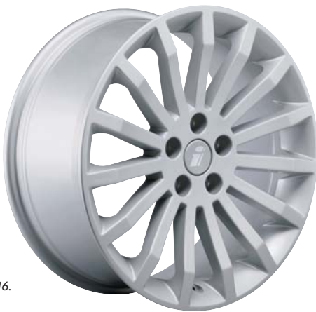
Light alloy wheel in Softstar design in the dimensions 6 x 15 up to 7 1/2 x 17.
